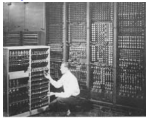
Examining a hot tube mount checking among ENIAC's 18000 positions.
